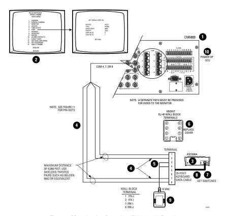
Figure 8. RS-485 Interface Connections (CM6800-48X8 Shown)
